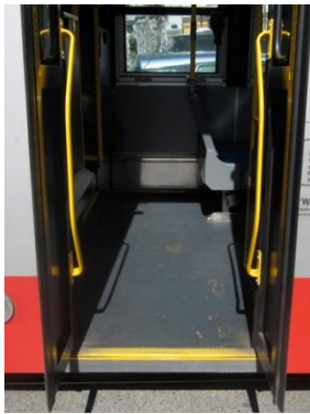
Buses with low floors speed up boarding time by reducing the number of steps required to board the bus.
