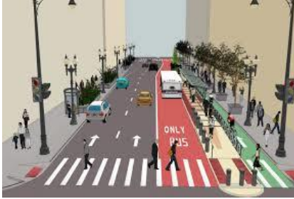
Bus-only lanes are an integral part of any BRT system, allowing buses to travel without being impeded by other vehicles
