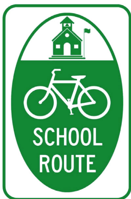
FIGURE 3-1. SCHOOL BIKE ROUTE SIGN
