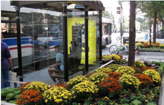
Sufficient sidewalk width is necessary to allow for pedestrian amenities, such as bus shelters, without impinging on circulation. Michigan Avenue, Chicago.
