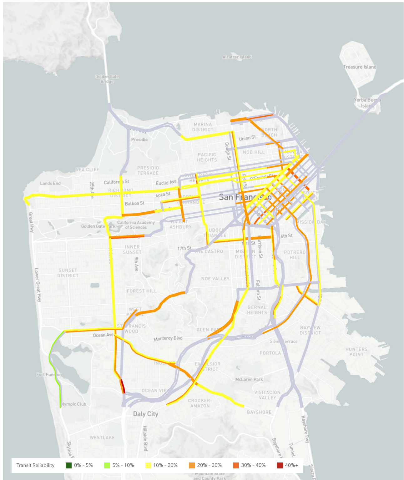
Figure 4-9: 2019 Average Muni Bus Speed Variability on CMP Network Segments, Weekday AM Peak
