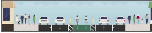
PROPOSED CROSS SECTION FOR VALENCIA WITH 15 FT. SIDEWALKS VALENCIA STREET FROM 15TH TO 19TH STREETS
