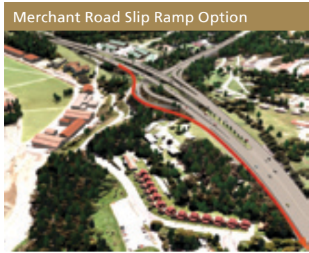
Merchant Road Slip Ramp Option This option would provide a new direct connection from westbound Doyle Drive to Merchant Road and improve access to the Golden Gate Visitors' Center
