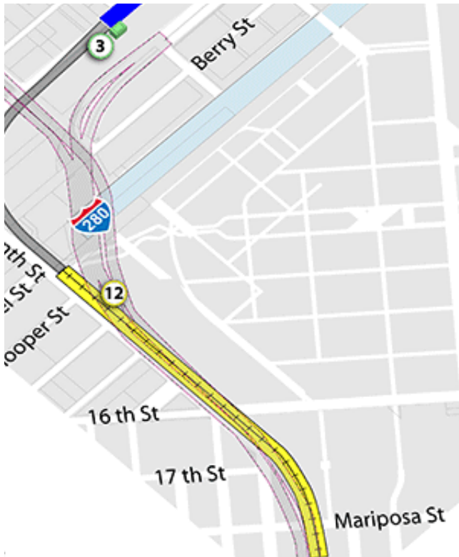
Exhibit 17: Turnback Track as identified in DTX SEIS/R
