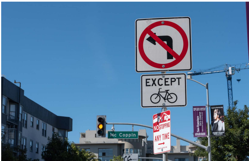
Figure 3-6. Turn restrictions can reduce potential conflicts thus improving safety for pedestrians and bicyclists.
