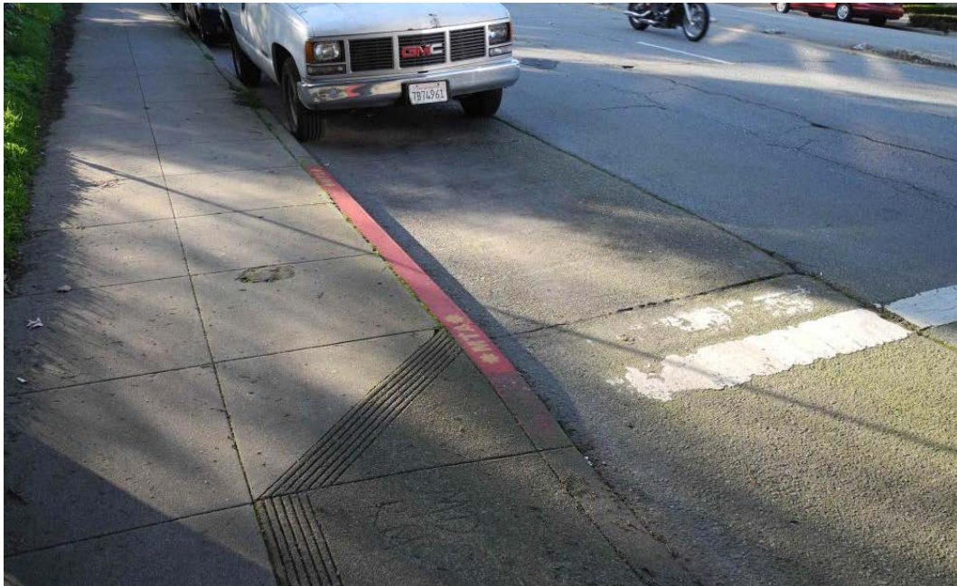
Figure 3-9. Daylighting improves pedestrian visibility at crosswalks and corner intersections but may require the removal of a parking space.
