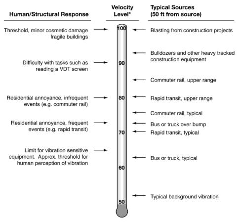
\* RMS Vibration Velocity Level in VdB relative to 10<sup>-6</sup> inches/second
