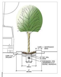
Under Build Alternative 3, vegetated swales could potentially be incorporated in one of the center medians to capture stormwater runoff from the transitway and could potentially infiltrate some of the runoff into the ground.
