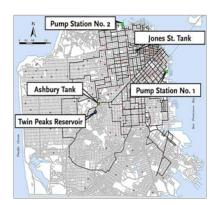
The auxiliary water supply system (AWSS), constructed after the 1906 earthquake, is a water distribution system operated and maintained by the San Francisco Fire Department. It delivers water under high pressure for fire fighting and is independent from San Francisco's domestic water system. It consists of 2 pump stations, 2 water storage tanks, 1 reservoir, 172 cisterns, and approximately 135 miles of pipes.
